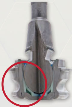
OEM BALL JOINT Plastic bearing with sealed design
